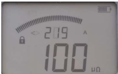
Max current during test was 219 A.
