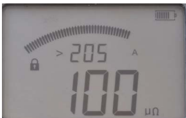
Min current during test was 205 A
